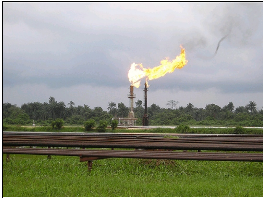
Figure 8 Throughout the world at oil and gas fields and refineries, gas is “flared,” or burned. This wastes a precious resource and creates air pollution. It could be captured and stored, or converted to methanol, a liquid fuel that can easily be transported, even from remote regions such as this one in Nigeria. (Source: claimatelaw.)
