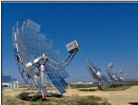
Figure 18 To make small amounts of electricity—for villages, islands and other remote places, for example—a saucer-shaped mirror focuses sunlight onto a Stirling engine, which drives a small generator to make electricity. The engine is roughly the size of a 55-gallon barrel.
