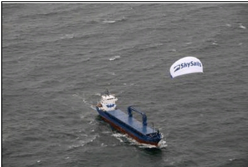
Figure 3 Beluga Shipping and SkySails have teamed to develop the use of giant kites as auxiliary power—a kind of hybrid wind/fossil-fuels system. The ship MV Beluga went from Germany to Venezuela in early 2008, a total of 11,952 nautical miles using this 160-square-meter kite to supply roughly 20 percent of the engine's power. The next step is to double the kite's size, which is predicted to save $2000/day in fuel costs. (Source: New Scientist)
