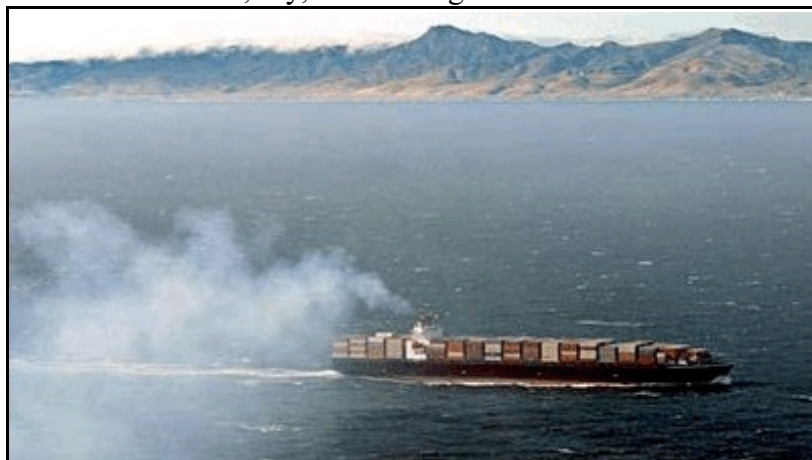
Figure 1 International shipping burns only between 2 to 4 percent of the world's fossil fuels each year, but accounts for more than 5 percent of the global \text{NO}_x emissions and more than 14 percent of the global sulfur emissions from human activity.
